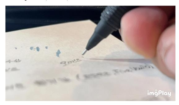
Semi-automatic mechanical pencils, such as the Pentel Orenz Nero, Orenz AT, and Pilot S30, have a spring built into the nib (sleeve). This spring automatically adjusts the lead length by retracting and retracting as the lead wears. This subtle movement repeats as you write, giving the illusion of continuous lead ejection.
