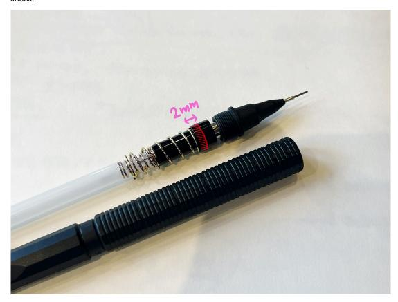
The cut-off part must be neatly trimmed to the same thickness as the back part to ensure that the spring can move properly and does not get caught inside the barrel.
