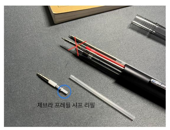
Cut the connecting part of the multi-pen's mechanical pencil unit (circled in the photo) to approximately 1.2mm.
