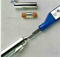
To store away the fineline holder, release the lead clutch by pressing push-button and simultaneously push protector sleeve back into writing point with finger. Refilling MARS fineline holders is easy. The push-button is removed and about six leads are poured into the feed chamber from the MICROGRAPH fineline lead refill tube.
